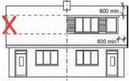
Box dormer extension on small semi-detached house (in this case it is permissable to build up to the party wall) Dormer should not extend out to verge
